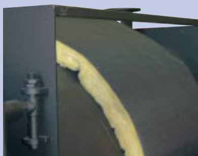
High-density glass wool thermal insulation, 80 mm thick.
